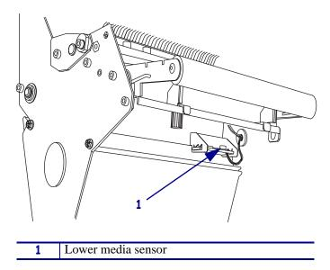
**2.** Slide the lower sensor until it is under the upper media sensor. Gently pull wires out as needed (wires should have a little slack).
